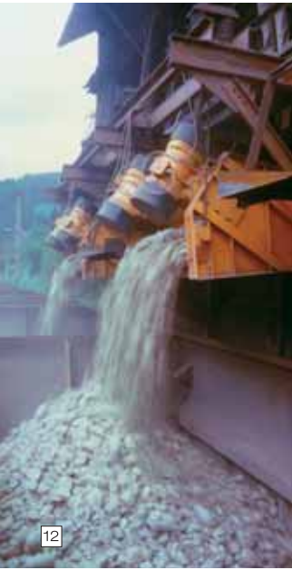
11 Regelbare Unwuchtrinne Unbalance motor feeder with stepless capacity adjustment
